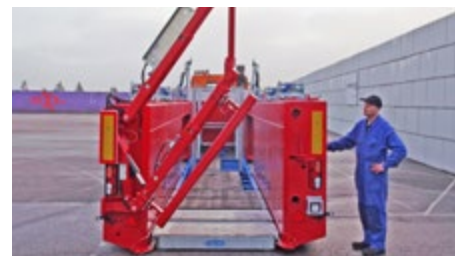
Hydraulic multifunctional back door, can be pivoted horizontally/vertically and is width-adjustable (standard with PrefaMAX-A).
