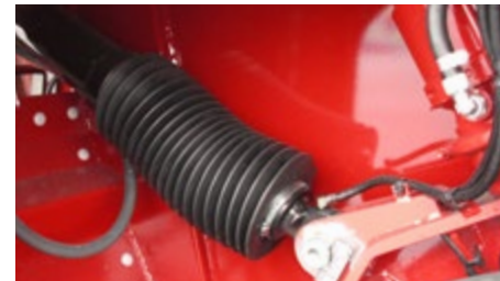
Standard equipment: Protection jackets on the hydraulic cylinders
