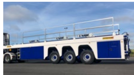
Removable hand rail on the lateral beams
