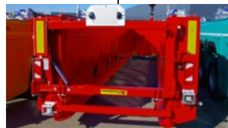
Vertically adjustable rear door, hydraulically activated
