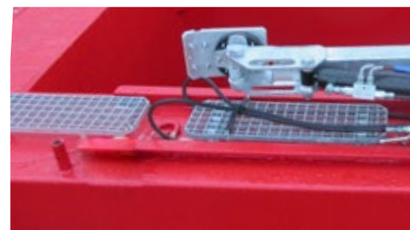
Standard equipment: Serrated floor on the lateral beams
