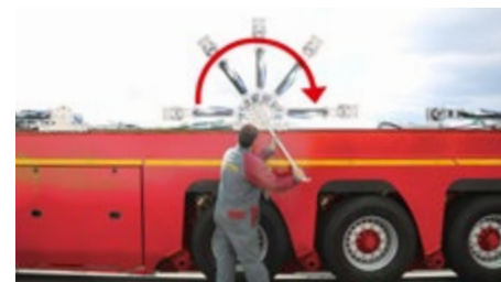
Handling of the load securing systems easily carried out from the ground
