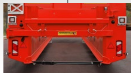
Cross-bar at the rear with eccentric closing
